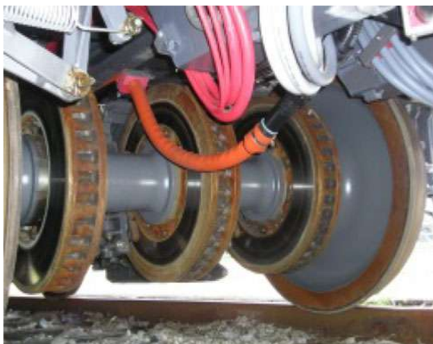
Fig. 3 Brake disks on trailer bogie
